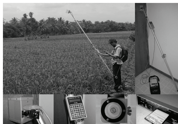
Fig. 2. Acquisition of spectral reflectance data in a paddy field at Bukateja village, Indonesia using a multispectral radiometer (MSR16R) left to right: sampling site, system spectroradiometer MSR16R, data logger controller (DLC), nivo, CT100 controller and head radiometer source: own research
