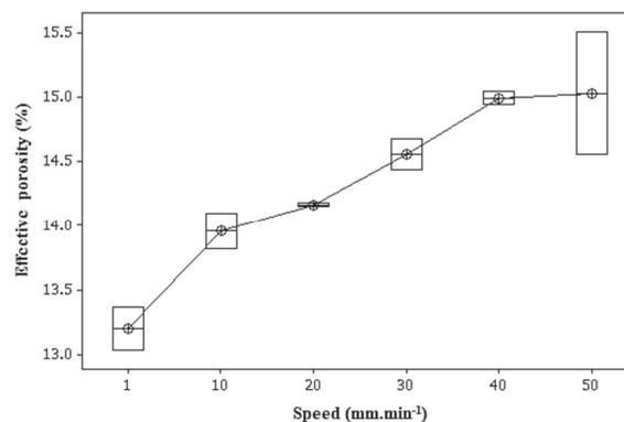
Fig. 4. Dependency between effective porosity (%) and compression speed ( $\text{mm}\cdot\text{min}^{-1}$ ) of jatropha bulk seeds
