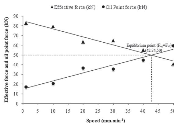
Fig. 6. Linear relationship between effective force and oil point force with different compression speeds
