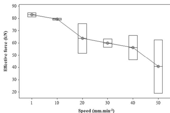
Fig. 5. Dependency between effective force and compression speed ( $\text{mm}\cdot\text{min}^{-1}$ ) of jatropha bulk seed
