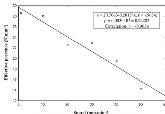
Fig. 8. Relationship between effective pressure and compression speed
