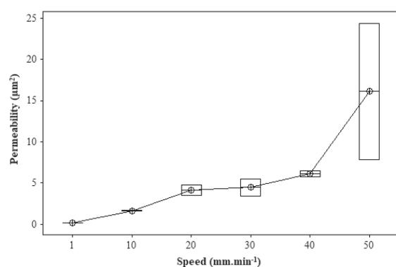
Fig. 7. Dependency between permeability ( $\mu\text{m}^2$ ) and compression speed ( $\text{mm}\cdot\text{min}^{-1}$ ) of jatropha bulk seeds
