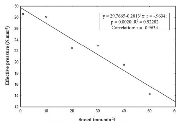
Fig. 8. Relationship between effective pressure and compression speed
