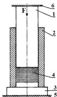
Fig. 1. Scheme of used laboratory briquetting press
