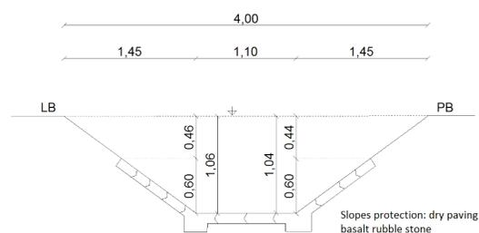
Fig. 1. Cross-section profile of the Pyský brook (values in m)
