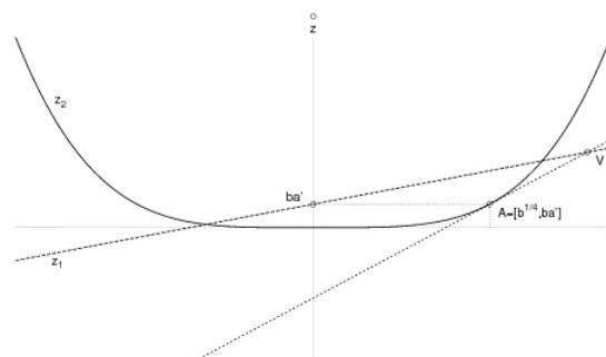
Fig. 4. Chart showing the gradual approximation of the intersection of the function  $z_2$  and the line  $z_1$ . The first approximation is the point A, the second is the point V
