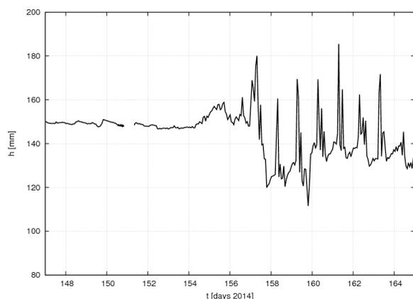
Fig. 2. Water level fluctuation of the Pyský brook before and after the algae layer removal (on the 155th day of the year, i.e. on June 4th, 2014). After using the formula for flow rate ( $Q = S v$ ) and data from the velocity profile measurement using balls (Dvorková, Zeman, 2013) we found that the median level for this measured episode corresponds to  $80 \pm 6$  l s<sup>-1</sup>
