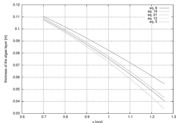
Fig. 5. Comparison of various functions depicting the dependence of the algae layer thickness on the velocity of water flow in the Pyský brook channel. The results obtained by the equations (12) and (19) are very similar. Their functions (curves) nearly overlap in the graph.
