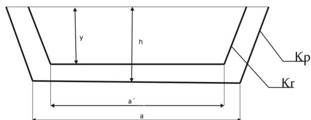
Fig. 3. Scheme of the channel with the algae layer
