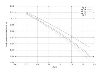
Fig. 5. Comparison of various functions depicting the dependence of the algae layer thickness on the velocity of water flow in the Pryský brook channel. The results obtained by the equations (12) and (19) are very similar. Their functions (curves) nearly overlap in the graph.
