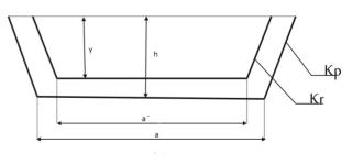
Fig. 3. Scheme of the channel with the algae layer Kp = original channel, Kr = channel with reduced discharge
