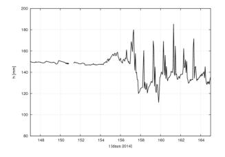
Fig. 2. Water level fluctuation of the Pryský brook before and after the algae layer removal (on the 155th day of the year, i.e. on June 4th, 2014). After using the formula for flow rate (Q = S v) and data from the velocity profile measurement using balls (D v o r a k o v a, Z e m a n, 2013) we found that the median level for this measured episode corresponds to  $80 \pm 61 \text{ s}^{-1}$
