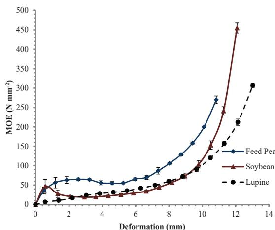
Fig. 4. Moduli of deformation of feed pea, soybean, and lupine at 9% moisture content, gradually compressed to 100 kN
