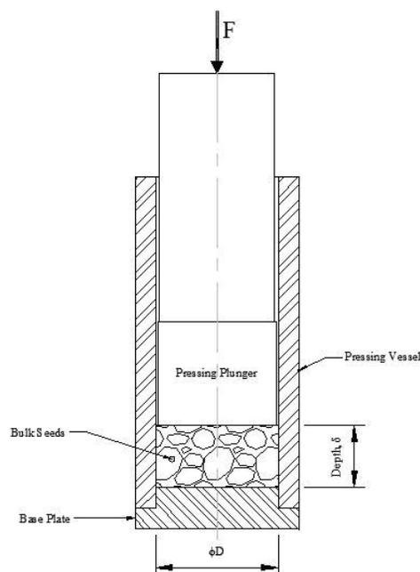
Fig. 1. Schematic view of the experimental setup
