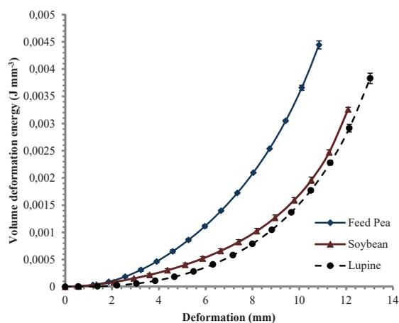
Fig. 3. Changes in volume energy demands with incremental deformation of bulk feed pea, lupine, and soybean seeds at ≈ 9% moisture content, loaded gradually to 100 kN
