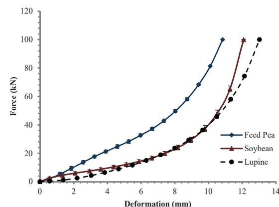
Fig. 2. Measured mechanical characteristics of the selected crops at moisture contents of ≈ 9% (dry basis) and crushing depths of 30 mm
