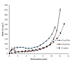
Fig. 3. Changes in volume energy demands with incremental deformation of bulk feed pea, lupine, and soybean seeds at  $\approx 9\%$  moisture content, loaded gradually to 100 kN
