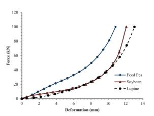
Fig. 2. Measured mechanical characteristics of the selected crops at moisture contents of  $\approx$  9% (dry basis) and crushing depths of 30 mm
