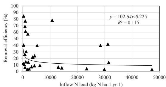
Fig. 8. Relationship between inflow nitrogen load (kg N ha<sup>-1</sup> per year) and treatment efficiency (%) in constructed wetlands treating agricultural drainage waters
