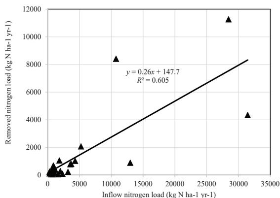
Fig. 7. Relationship between inflow and removed nitrogen loads (kg N ha<sup>-1</sup> per year) in constructed wetlands treating agricultural drainage waters
