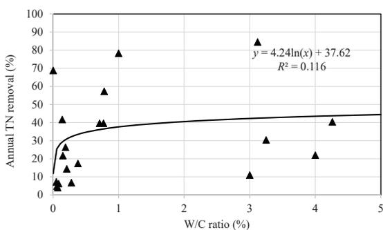
Fig. 6. Dependence of total nitrogen (TN) removal efficiency (in %) of the constructed wetland on the constructed wetland (W)/drained catchment (C) area ratio (in %)
