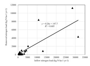
Fig. 7. Relationship between inflow and removed nitrogen loads (kg N ha-1 per year) in constructed wetlands treating agricultural drainage waters
