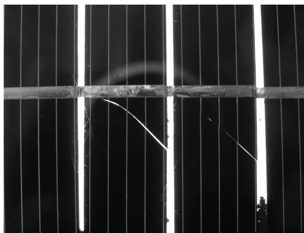
Fig. 2. Detail of the damaged place in the visible spectrum
