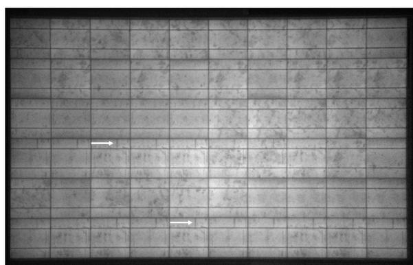
Fig. 3. Image of electroluminescence of a larger undamaged photovoltaic panel
