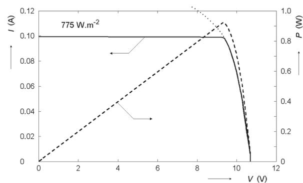
Fig. 5.  $V-I$  and  $V-P$  characteristic of a photovoltaic panel during autumn season with solar radiation intensity of  $775 \text{ W m}^{-2}$
