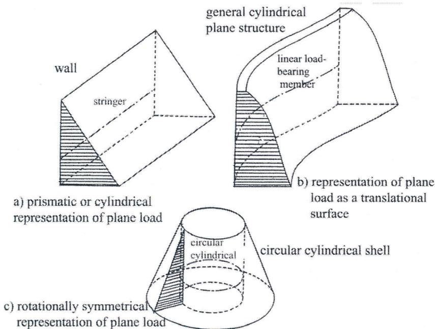
Fig. 1. Character of examined plane structures with linear load-bearing members and the types of their all-surface loads (some typical examples)
