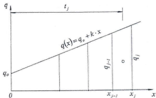
Fig. 3. Linearly increasing load  $q(x) = q_0 + k \cdot x$  uniformly distributed to stringers for  $n = 4$
