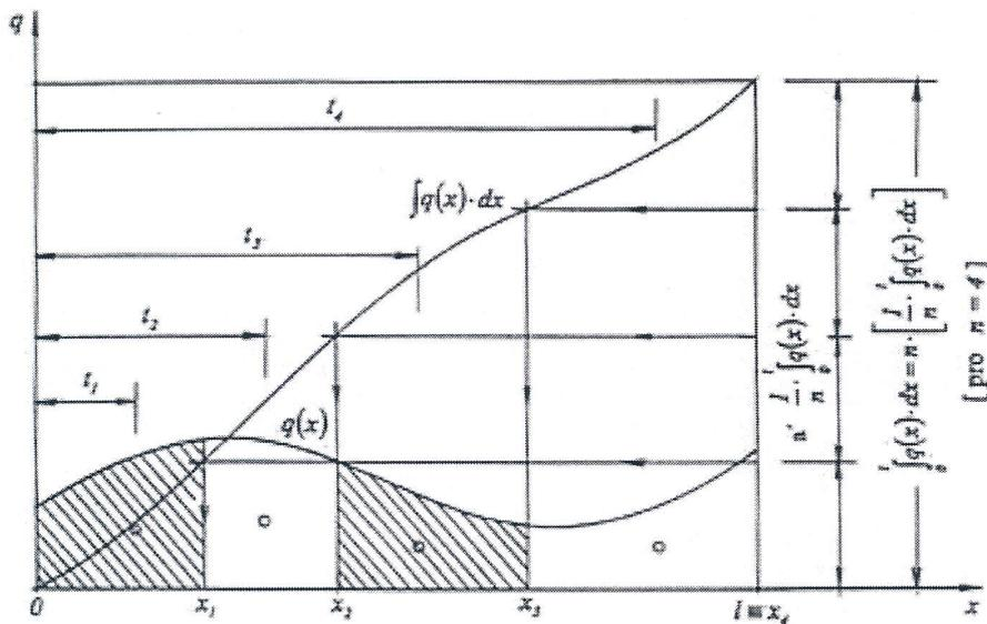
Fig. 2. Load  $q(x)$  uniformly distributed to stringers for  $n = 4$
