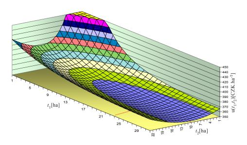
$t_1$  – operating time up to first chisel replacement (ha),
