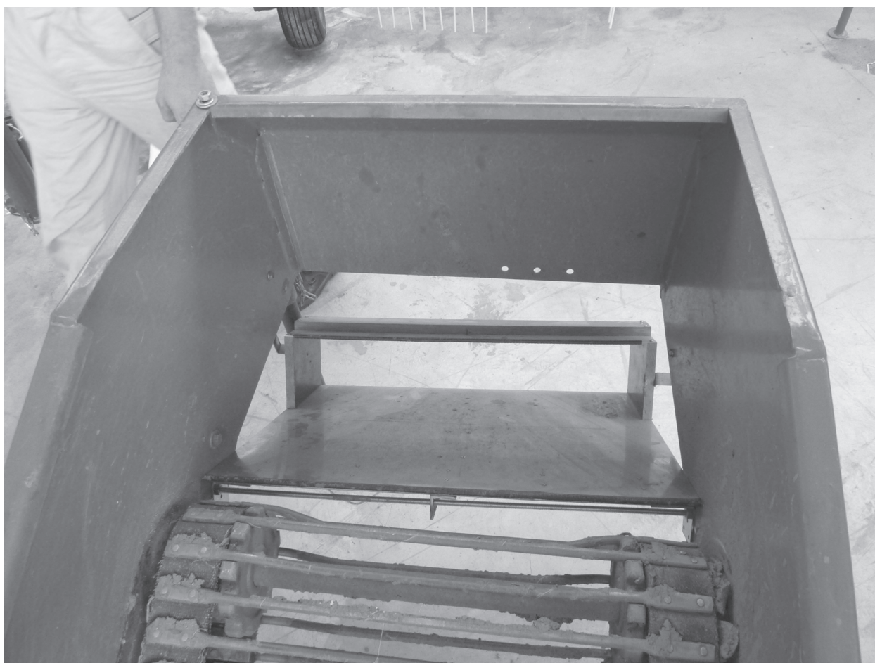
Figure 1. The view of parallel plate capacitive throughput sensor integrated to one row conveyor potato digger Akpil (Akpil Co., Poland)
