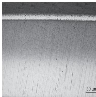
Fig 2b. TiN coating on nitrided surface light microscope (angled section)
