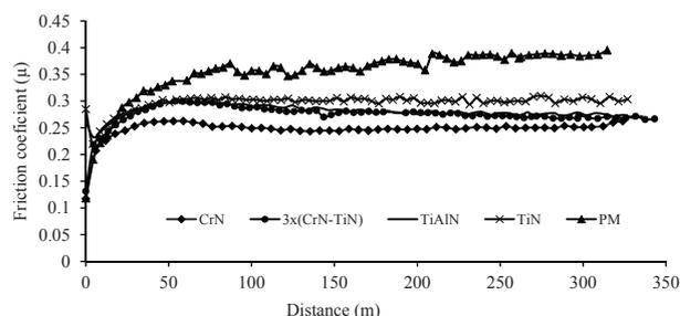
Fig. 7. Friction coefficient dependent on distance at 22°C and load 5 N
