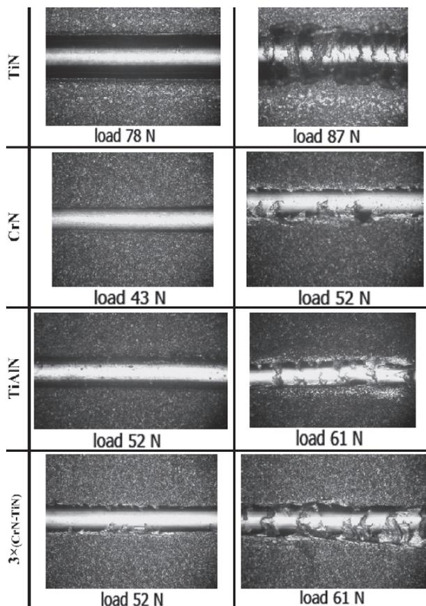
Fig 4. Results of the coating adhesion by a scratch test (indicated forces are maximum loads in given locations, magnifications is 50 x )
