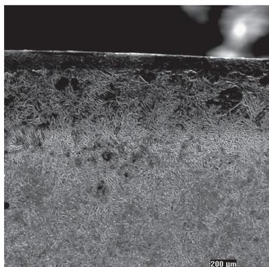
Fig 2a. TiN coating on nitrided surface SEM
