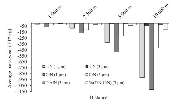
Fig. 9. Average mass wear dependent on distance under load 150 N
