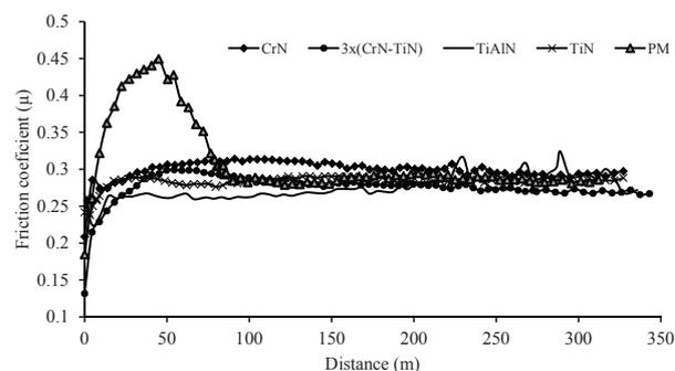
Fig. 8. Friction coefficient dependent on distance at 350°C and load 5 N
