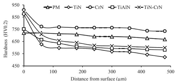
Fig 5. The hardness of nitride layer on measured samples. (Hardness of coatings was not measured)
