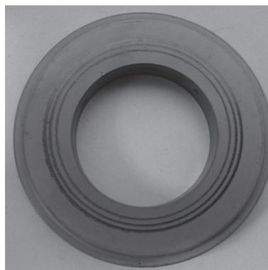
Fig 1b. Specimen with PVD coating TiAlN
