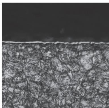
Fig 2c. TiN coating on nitrided surface light microscope (magnification 500 × – cross-section)
