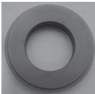
Fig 1a. Specimen with PVD coating TiN
