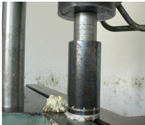
Fig. 2. Pressing vessel with plunger and a caked kernel oil
