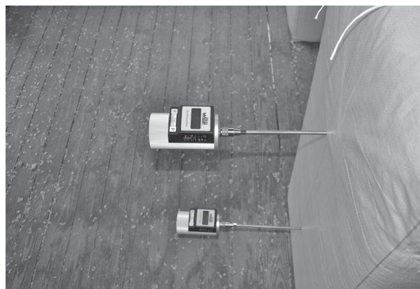
Fig. 2. Measurement of hop moisture content in a bale
