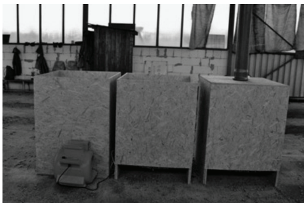
Fig. 1. Storage container with active ventilation (on the left), with passive ventilation (on the right) and check container (in the middle)
