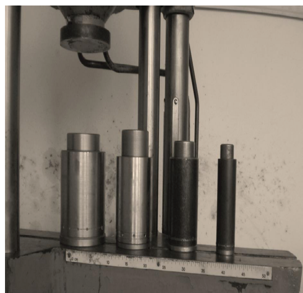
Fig 1. Compressive device and vessel diameters 100, 80, 60 and 40 mm with plungers.
