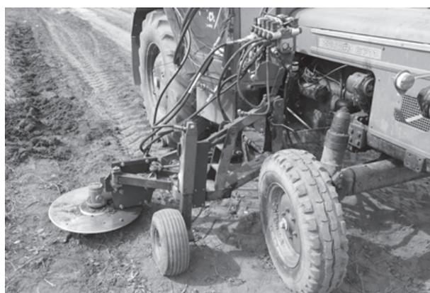
Fig. 5. Experimental model of mechanical pruner
