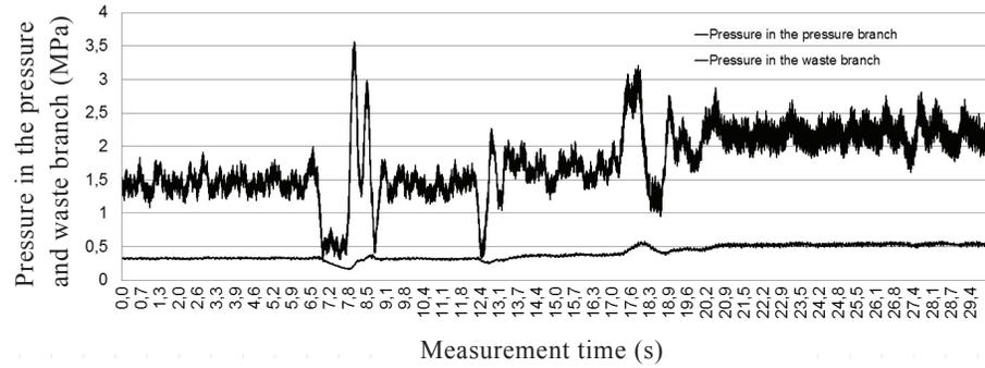
Fig. 7. Pressure at the input and output depending on time of 50 mm recess
