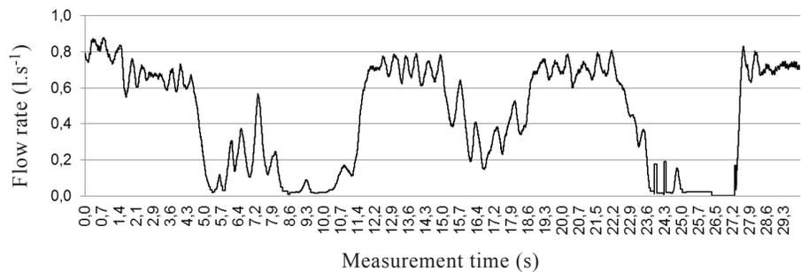
until the time when the cutting disc was dug out just below the hop-field surface. The hydraulic oil pressure in the pressure branch subsequently levelled off at the value of 5 MPa. The flow curve in the pressure branch, recorded in the course of the measurement (Fig. 8), also corresponds to this development.
