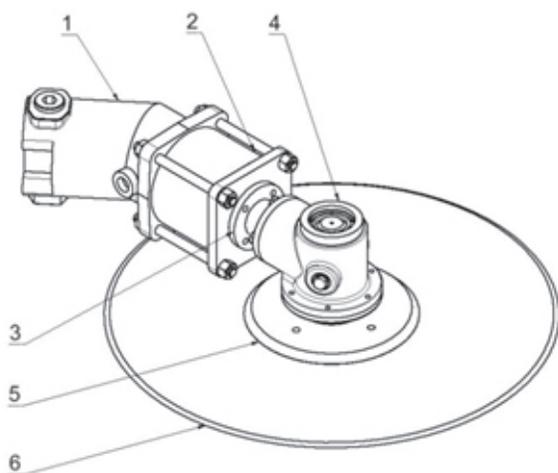
Fig. 1. Rear transmission with hydromotor
