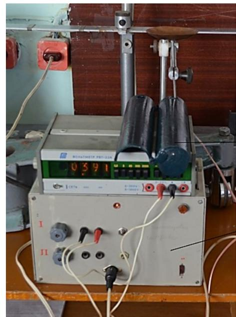
Fig. 4. Plating device for measuring the stressed state of the plane: 1 - tensor station; 2 - device. Voltmeter and strain gauge RV7-22A, produced in Russia (Special cable bureau)
